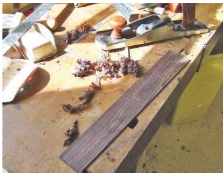
▲ Pic.21 Plane the rosewood fingerboard to size and cut fret slots using a tenon saw and a block of timber as a fence to give accurate, square cuts
